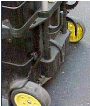
Figure 3 Uneven, thinning wheels on a hand truck
